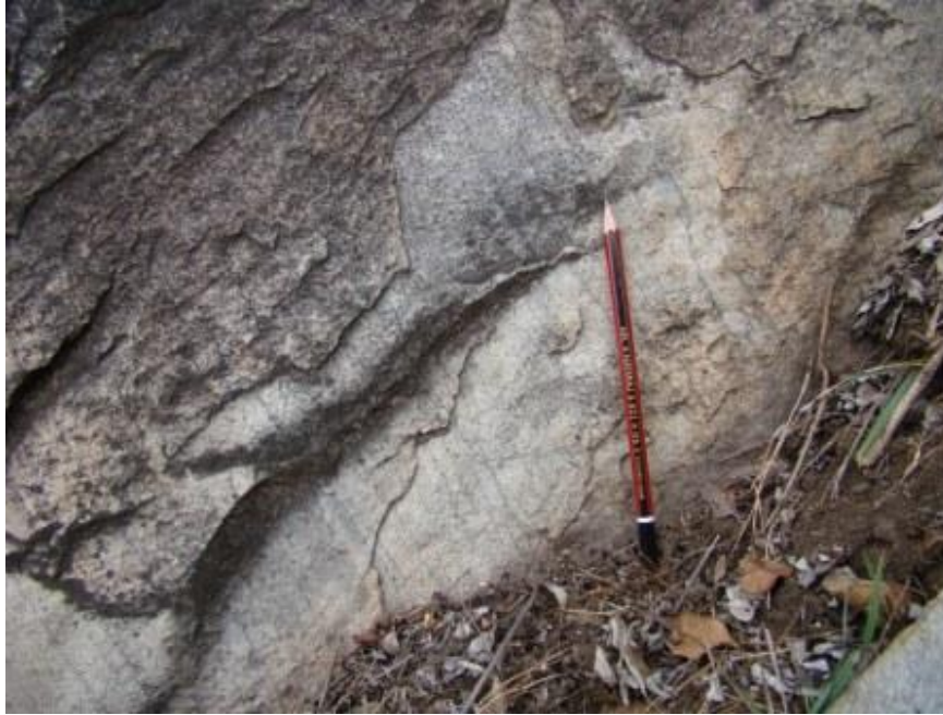
Fig 26 Thin layers of foliated Meta basic rocks near the western portal area.
